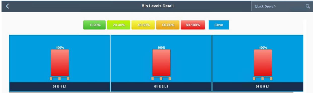
You will see at the top of the display, the color guide which indicates the % level the bin is currently at.
